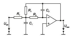
$$C_1 = 100 \text{ nF}; C_2 = 15 \text{ nF}$$
