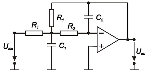
$$C_1 = 100 \text{ nF}; C_2 = 15 \text{ nF}$$
