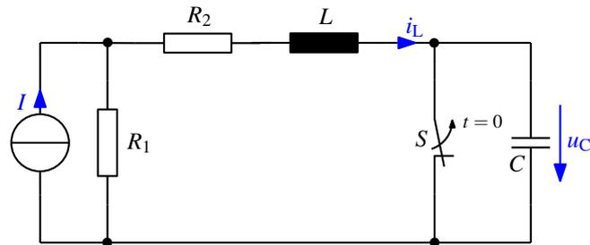
$$R_1 = 5\Omega, R_2 = 10\Omega, L = 2\text{mH}, C = 100\text{nF}, I = 3\text{A}$$
