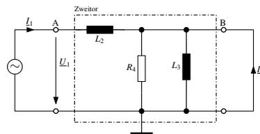
$$\underline{H}_{11} = \left. \frac{\underline{U}_1}{\underline{I}_1} \right|_{\underline{U}_2=0} = j\omega L_2 \tag{18}$$
