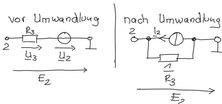
$$\Rightarrow E_2 = \underline{U}_3 + \underline{U}_2 \quad \Rightarrow \underline{U}_3 = E_2 - \underline{U}_2$$
