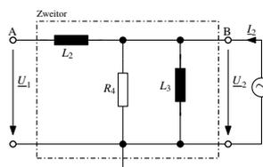
$$\underline{H}_{12} = \left. \frac{U_1}{U_2} \right|_{I_1=0} \quad \text{mit } U_1 = U_2 \Rightarrow \underline{H}_{12} = 1 \quad (20)$$
