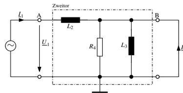
$$\underline{H}_{11} = \left. \frac{\underline{U}_1}{\underline{I}_1} \right|_{\underline{U}_2=0} = j\omega L_2 \quad (18)$$
