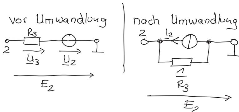
$$\Rightarrow \underline{E}_2 = \underline{U}_3 + \underline{U}_2 \Rightarrow \underline{U}_3 = \underline{E}_2 - \underline{U}_2$$
