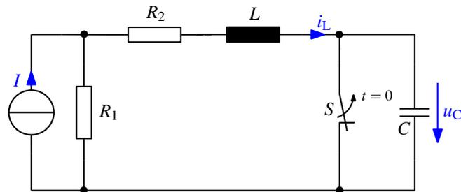
$$R_1 = 5\Omega, R_2 = 10\Omega, L = 2\text{mH}, C = 100\text{nF}, I = 3\text{A}$$
