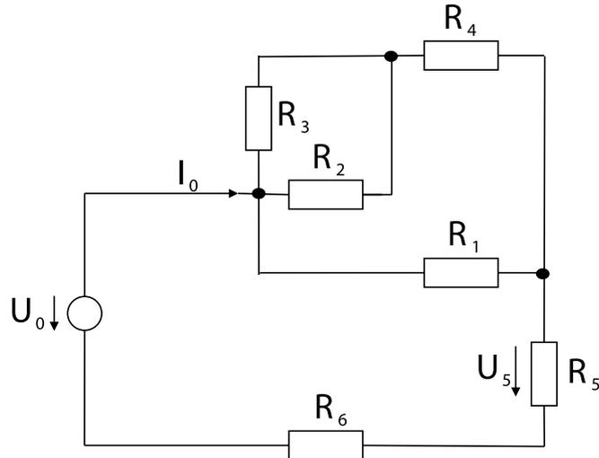
$$R_1 = R_2 = R_3 = 10 \quad R_4 = 5 \quad R_5 = 1 \quad R_6 = 4$$
