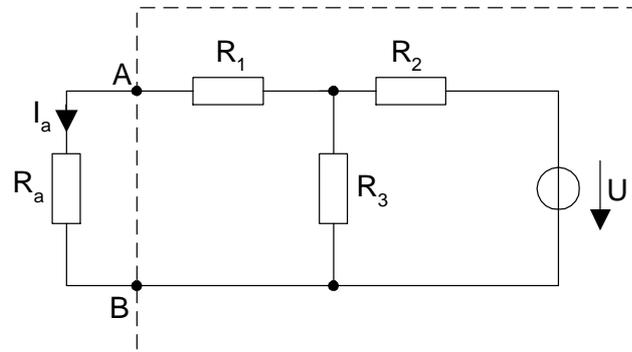
$$U = 10V; \quad R_1 = 1,5k\Omega; \quad R_2 = 3k\Omega; \quad R_3 = 1k\Omega; \quad R_a = 2,2k\Omega$$
