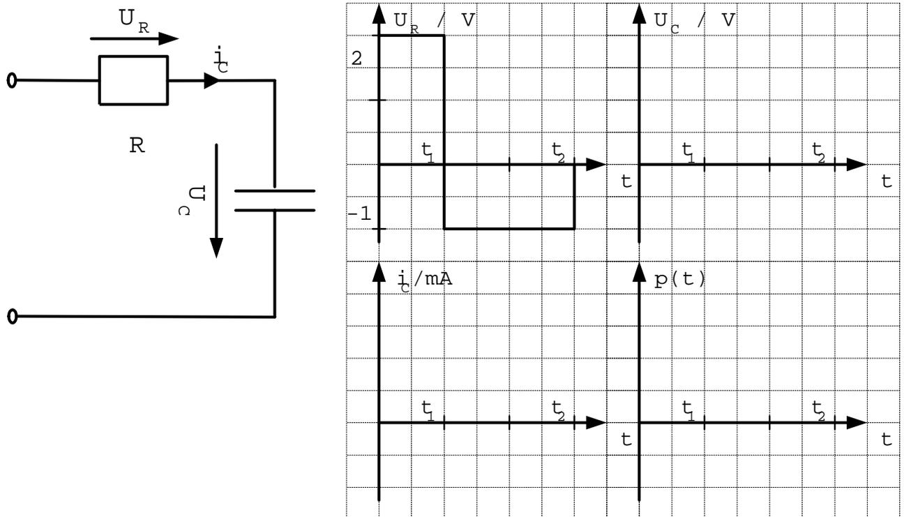
$$R = 1K\Omega, C = 100nF, t_1 = 1ms, t_2 = 3ms, U_C(t = 0) = 0$$
