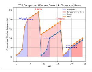
$$Throughput_{mean} = \frac{3}{4} \cdot \frac{cwnd[bytes]}{RTT[s]}[bytes/sec]$$
